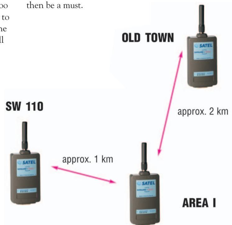
Location of the stations equipped with SATEL radio modems
