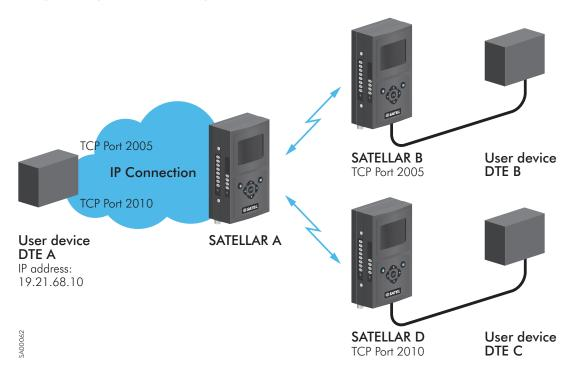
In this example the User device DTE A is capable simultaneously listen several ports. Both SATELLAR B and SATELLAR C are configured to send the messages to User device DTE A, but to different ports. Following configuration is set to SATELLAR B and SATELLAR D, when User device DTE A has IP address 192.168.1.1:
