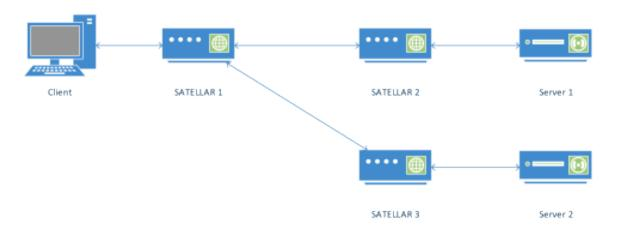
An example of how to use the proxy will be presented here. A network consists of 3 SATELLAR devices, one client and two servers. The IP addresses of the devices are as follows:
