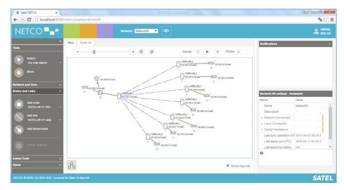
After the design process, NETCO provides a synchronization functionality to transfer modem settings from the NETCO to the radio modems one-by-one. Synchronization can be done locally over IP connection or over a USB cable. Local synchronization is often the case for the first time installation, after receiving the modem from the factory.
