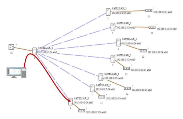
For the over the air (OTA), or field synchronization, NETCO software is first connected in a local manner to the master SATELLAR, and then the synchronization is forwarded by the master modem to the correct target device on the field. This also sets the requirement, that basic radio connectivity must be available i.e. the first synchronization of the devices has already been done.
