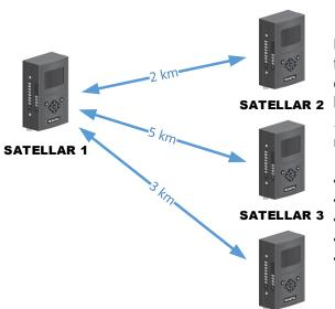
In this example there is a SATELLAR network consisting of four devices with RMAC addresses 1-4. ATPC needs to be enabled in the network, that each device gets at least RSSI between -85...-75 dBm. The ATPC is enabled in SATELLAR 1 first, and the starting transmit power of the device is 100 mW. ATPC is configured like this:
