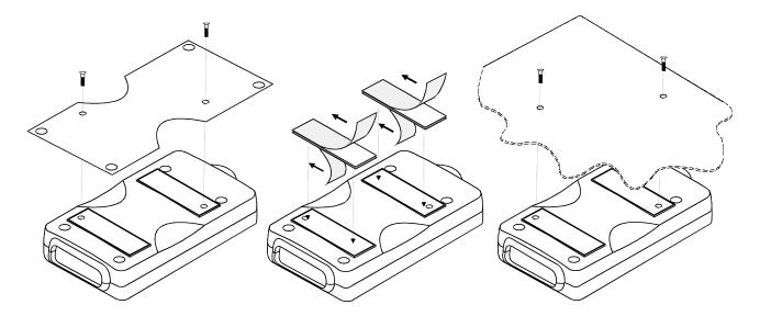
1. Installation with the installation plate supplied with the radio modem. The installation plate is fastened to the backside of the radio modem.
