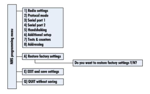
The original settings of the radio modem can be restored by selecting "A" in the Main menu and confirming "Y" (YES) on the prompt. By pressing any other button current settings will remain active. The modem will ask this question twice to make ensure that this is a valid command.
