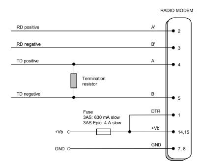
If the transmission lines are long the receiving end of the lines must be terminated using a separate termination resistor (typical values range from 100 -120 ohm depending on the characteristic impedance of the transmission line).
