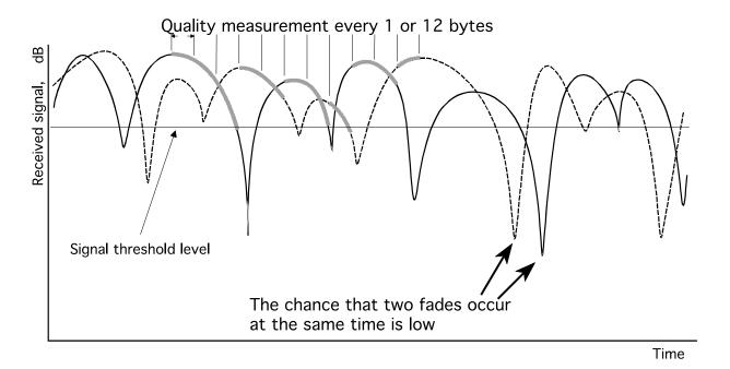
Received signals from two antennas. The selected signals are marked in grey.
