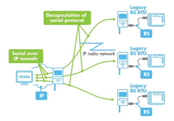
This kind of operation is enabled by the remote SATELLAR being able to output received protocol data from the serial port. Correspondingly SATELLAR IP router encapsulates responses from PLC serial port over the IP and then forwards responses towards the SCADA over IP.
