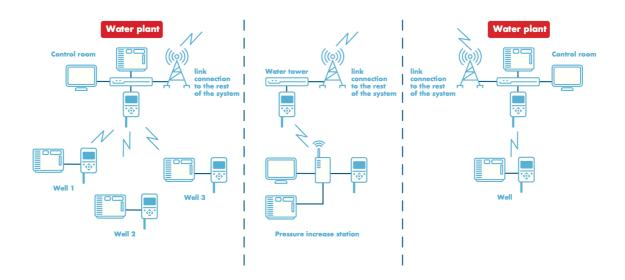
The control centre has a master radio modem router that delivers the messages to the sub stations. SATEL XPRS solution supports IP data transfer so no polling is needed. Management interface can be accessed with Internet browser. SATELLAR IP radio routers support many remote control protocols and are easy to combine to several direct control systems.
