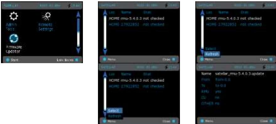
Figure 8.4 Firmware updater by CU: Graphical user interface (GUI/LCD)
