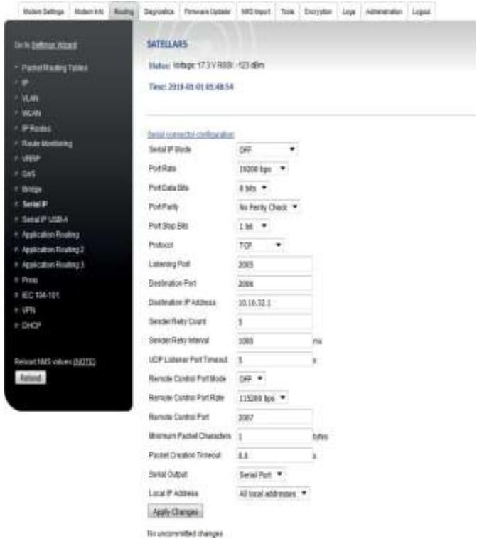
Figure 7.27 Configuration of Serial IP RS-232 via WWW-interface
