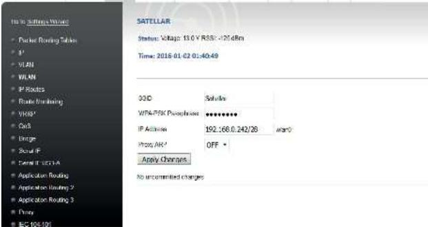
WLAN connection is configurable with parameters available at WLAN view. Available settings:
