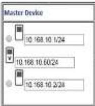
The redundant master consists of two physical devices using VRRP. Both devices need individual IP addresses, as well as a common virtual IP address that will be the IP address of the redundant master. The master settings need to be stored to two different devices.
