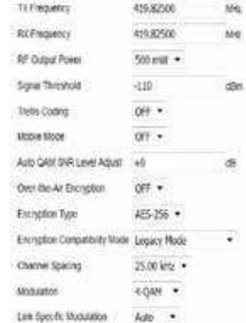
QAM-model settings page showing various parameters:
