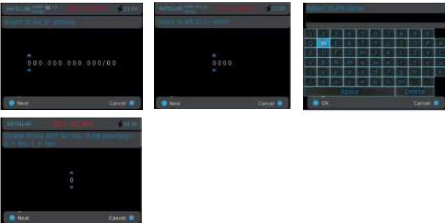
Figure 7.31 Configuring VLAN interface
