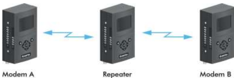
Network topology: Repeater Setting: Repeater
