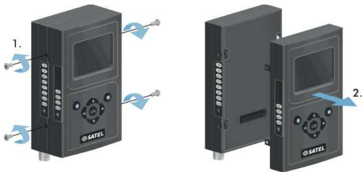
Figure 1.4 Modular construction, mounting of the central unit CU
