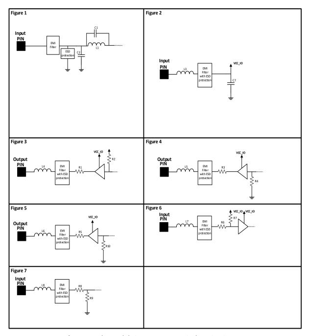
Figure 4.3 The module input-output equivalent circuits.
