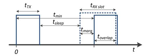
**Figure 6.1** Power save mode timing factors.
