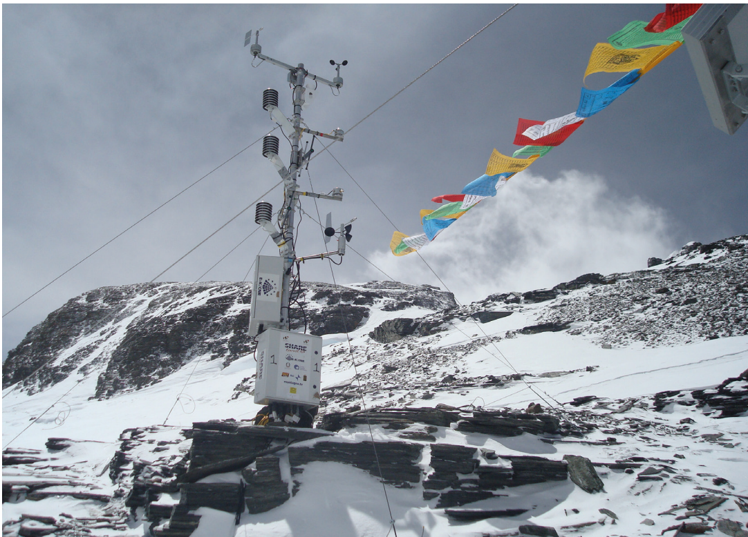
Everest region has several active weather stations in the range 4300 masl to 5700 masl. Their data is relayed to Pyramid through Kala Pathar's repeater station.
