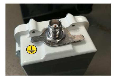
Besides the mains voltage safety, proper grounding is essential also for the error free operation of radio links and the protection against over-voltages and lightning. Although SATEL Proof radio modem incorporates a robust internal surge protection, the surge spikes and power transients caused by lightning, ESD or other electrical systems must be discharged to earth ground.
