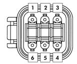
Pin-out of **Deutsch DT04-6P-CL09** power/data connector
