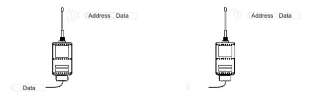
Reception addressing has been set ON and either the primary or secondary RX address of the radio modem is identical to the address of the received data packet.
