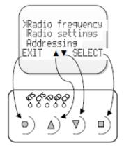
Pressing *DOWN* (▼) button the cursor moves downwards. Depending on the sub-menu, the button also scrolls the digits of numerical values when changing some settings.
