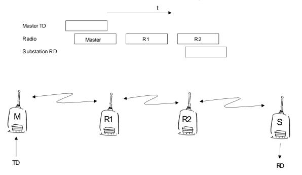
When using repeaters, the same packet is sent via a (radio) channel several times. A radio modem situated in the repeater chain will often hear other radio modems in addition to the immediate neighbouring radio modems. With *Source Mode Routing* the complete address information is sent
