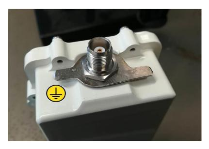
Besides the mains voltage safety, proper grounding is essential also for the error free operation of radio links and the protection against over-voltages and lightning. Although SATEL EASy-Proof incorporates a robust internal surge protection, the surge spikes and power transients caused by lightning, ESD or other electrical systems must be discharged to earth ground.
