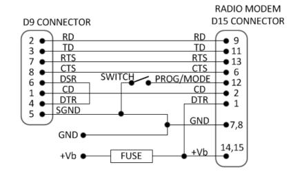
The wiring below is for configuring the radio modem via the Programming mode menu.
