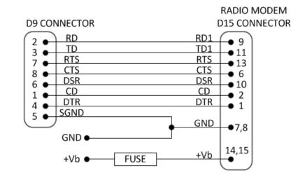
A typical connection between the Port 1 of the radio modem and the PC serial port (RS-232) using the handshaking signals is depicted in the schematic below.
