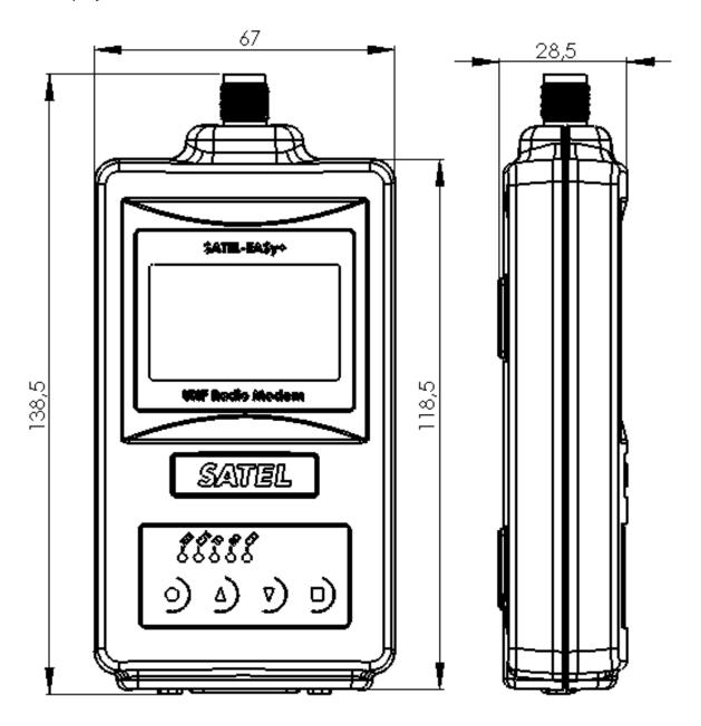
Figure 1.1 SATEL-EASy+ mechanical dimensions
