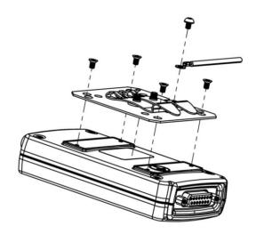
Figure 1.7 DIN rail installation plate
