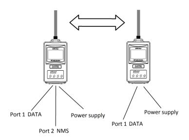
Figure 1.3 SATEL-EASy+ basic NMS set up
