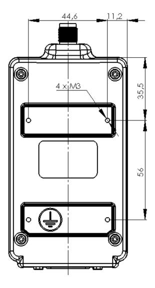
Figure 1.4 Mounting screw positions
