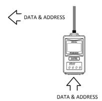
Transmission address has been set OFF. Radio modem will transmit the data packet as such. Transmission addressing has been set ON. The radio modem will add the primary TX address to the beginning of the data packet.
