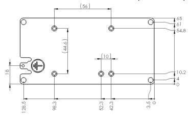
Figure 1.5 Installation plate and dimensions
