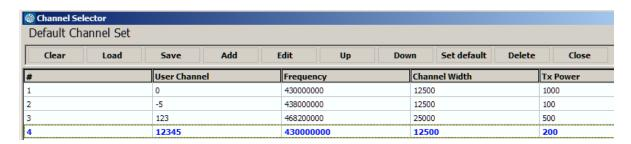
Entering to the Channel List -feature parameters require elevated access level to software tools, SATEL Configuration Manager and/or SATEL NETCO DEVICE. Please contact SATEL for additional information at <a href="https://www.satel.com/support-and-services/technical-support/">https://www.satel.com/support-and-services/technical-support/</a>
