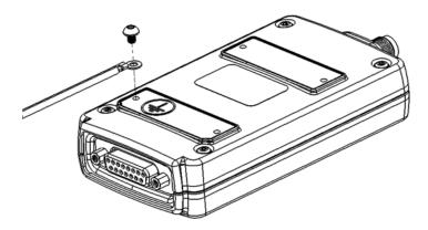
Figure 1.8 Grounding to the back of the housing
