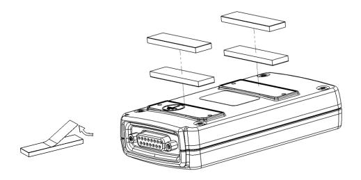
Figure 1.6 Velcro tape positions
