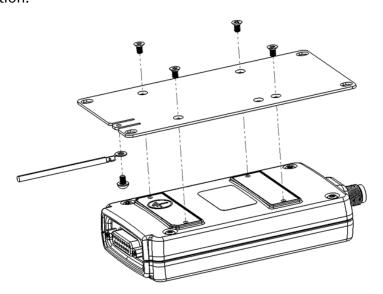
Figure 1.9 Grounding to housing
