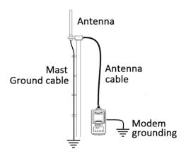
Figure 1.11 Grounding the antenna
