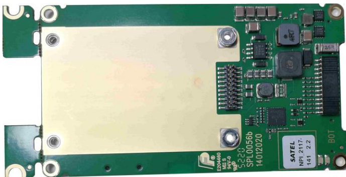
SATEL-B2 motherboard with the female horizontal 26-pin header connector (B2A variant)
