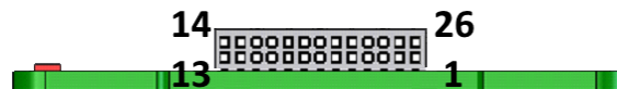
26-PIN HORIZONTAL FEMALE HEADER CONNECTOR (side view) on the bottom side at the end of the motherboard Part type: Weitronic 613-26-20-10-2-10 (2 x 13 pin, pitch 1.27 mm)
