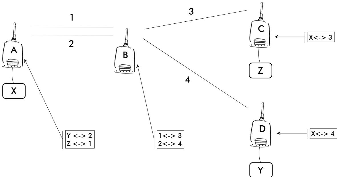
The above figure represents the same network, which has now been configured using the *Virtual Mode Routing*. The difference being that logical links are numbered instead of the radio modems. Operation is easy to understand by thinking of a telephone network realized with traditional overhead wiring.
