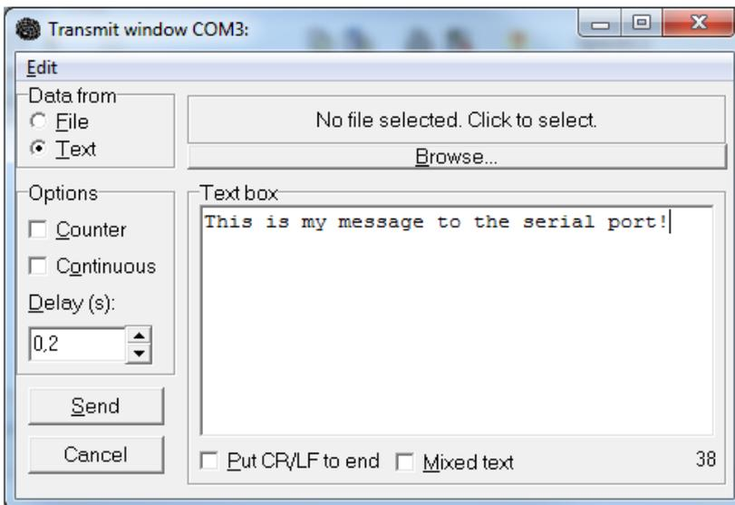
**Continuous** option should be selected if the transmission is to be repeated continuously, in which case the desired delay between packets should be entered into the **Delay** field. The **Counter** option will add a separate serial number to each sent packet. **File/Text** option is used to determine whether the text is to be sent from the **Text Box** window or from an open file. **Edit** selection contains the usual **Cut**, **Copy** and **Paste** commands.
