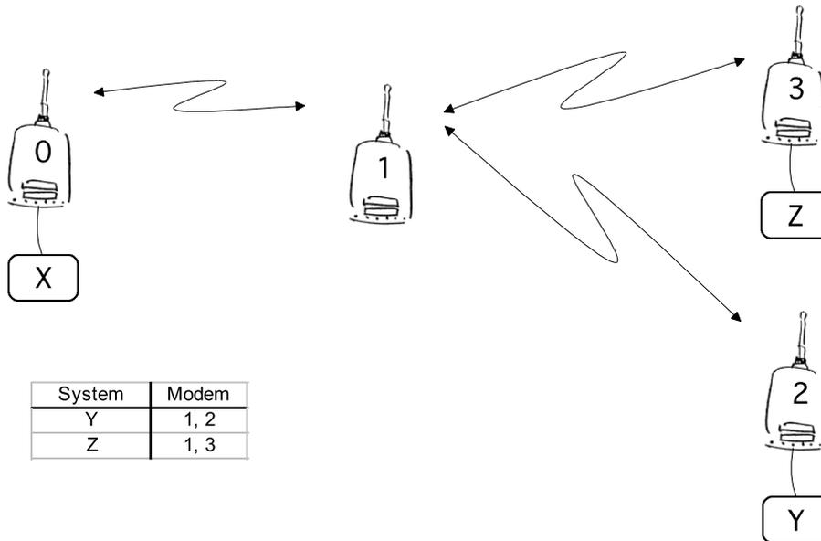
The above figure represents a network containing four (4) radio modems. Each radio modem is given a unique address (0...3). A terminal device has been attached to the three of the four radio modems and they communicate with each other using addresses X, Y and Z, respectively. Radio modem 0 and terminal device X together constitute the base station of the network and all routing information of the network has been programmed into this base station.
