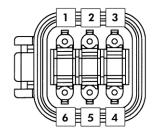
Pin-out of **Deutsch DT04-6P-CL09** power/data connector
